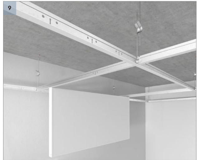
Rockfon Universal Baffles suspended between T24 profiles.
