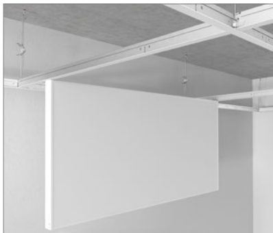
Rockfon Universal Baffle fixed between Chicago Metallic T24 profiles.
