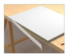
3. Align 5 mm overlap on front and press.
