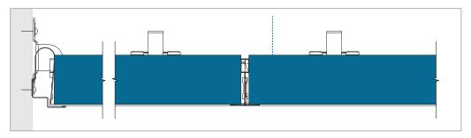
E-edge - Perimeter finish with wall angle trim and wall spring fixt. Wall spring fixt and the wall and bridging bracket are mandatory when cleaning and/or presure controle are required.
