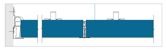
A-edge - Perimeter finish with wall angle trim and wall spring fixt. Wall spring fixt and the wall and bridging bracket are mandatory when cleaning and/or presure controle are required.
