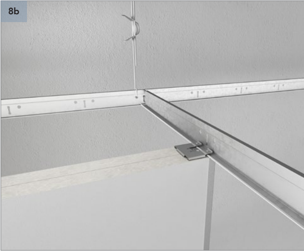
Fix Rockfon Industrial Baffle to the suspended T24 profiles. You can use the slots of the T24 profiles to align the baffles.
