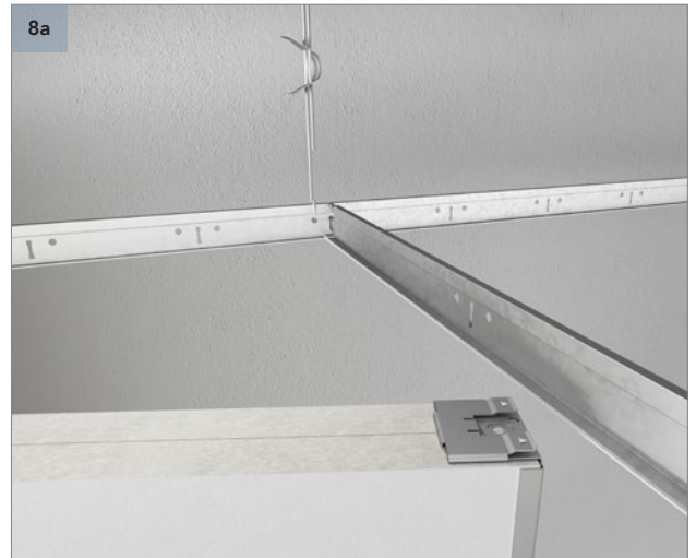
Fix the Rockfon Industrial Baffle to the suspended Chicago Metallic T24 grid.
